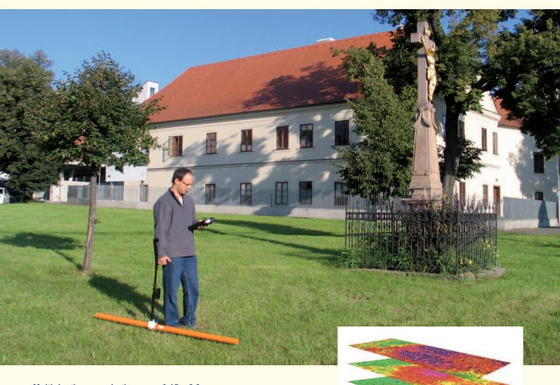
Multi depth survey in the range 0.15 - 2.3 mManual or continuous measuring modes with GPS
