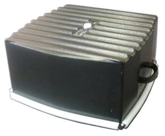
contains a pre-amplifier which is powered directly from the terraTEM console. The TRC sensors are designed to provide an equivalent reception to that of a 1000 square metre single turn receiver loop by compensating for their much reduced area with multiple turns of wire plus electronic pre-amplification.
