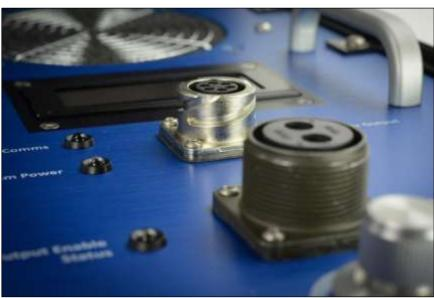
The 6 kW voltage rectifier **accepts either single or three phase input power**. Three phase power requires a suitable distribution board. Voltage output is either controlled from a front panel dial or via a serial connection with the terraTX-50 or terraTEM24 transmitters.
